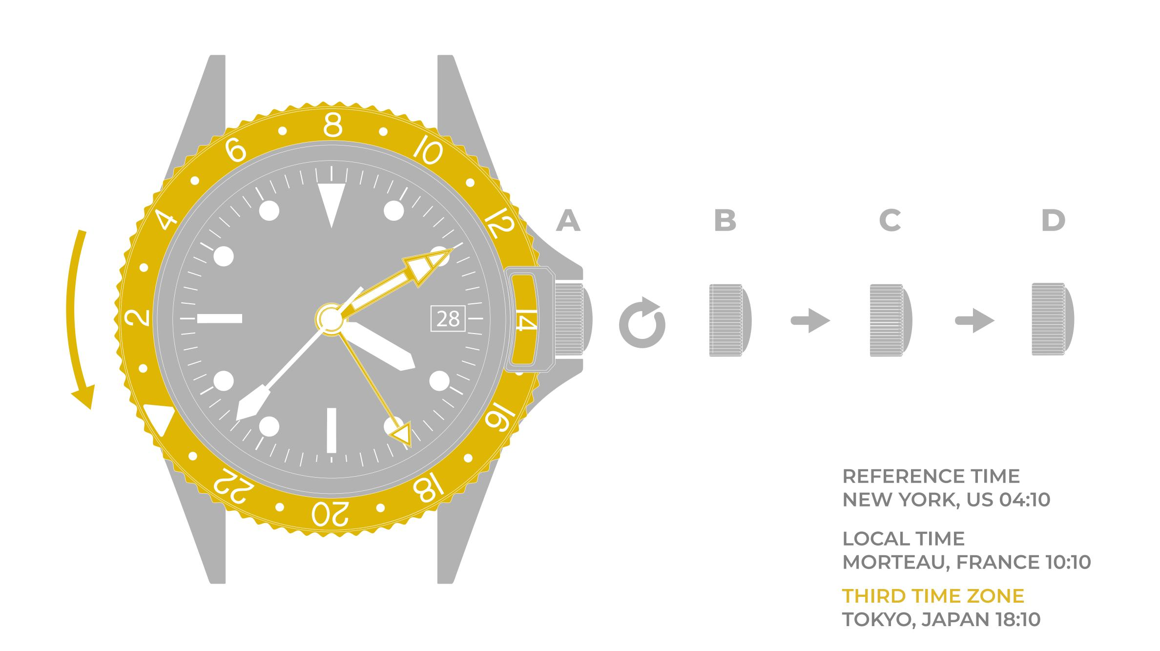
The unidirectional rotatable bezel allows precise measurement of dive times. For safety, the bezel rotates counter-clockwise only.
